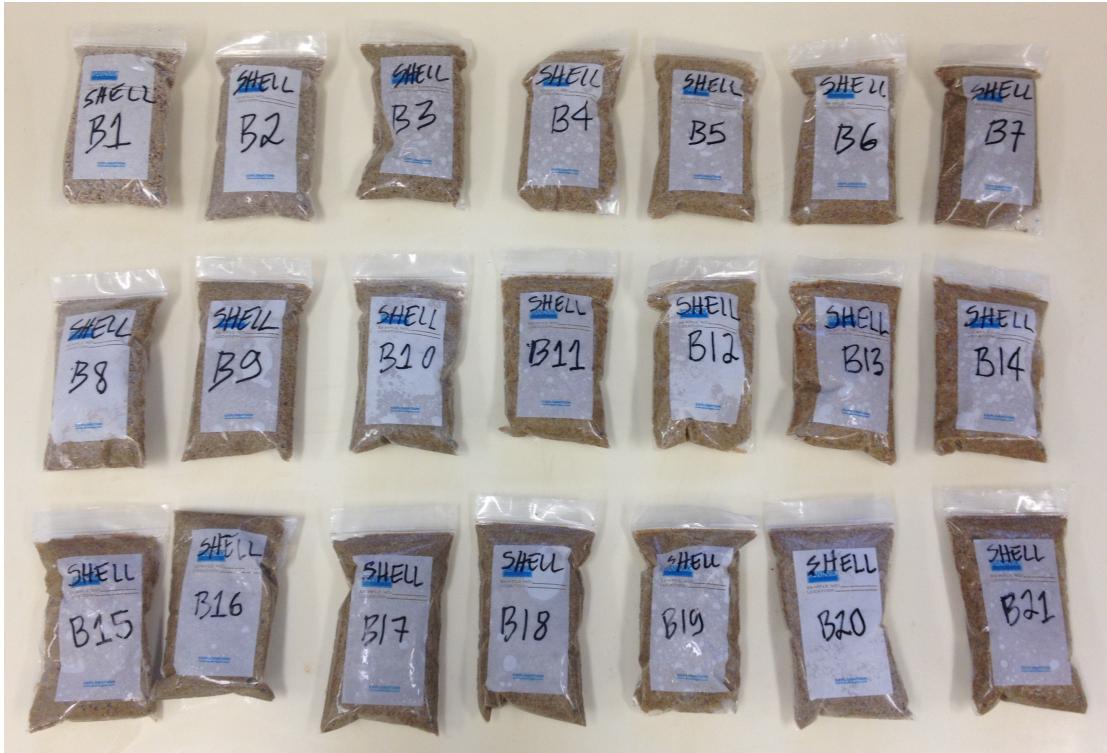
Fig. 7: Surficial beach sediment samples collected in the Illawarra Coast-South Compartment to be analysed for grain size and mineralogy
